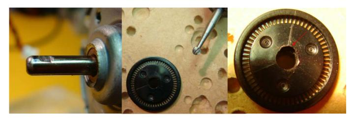
With a marker pen indicate the position of the sensor wheel on the motor shaft and then pull the wheel from the shaft.
